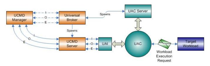
As you can see, Universal Command Agent for SOA gets its input from Universal Command through STDIN. When the parameters and data are passed in, the workload execution request is processed and any return data is passed back to Universal Command.
