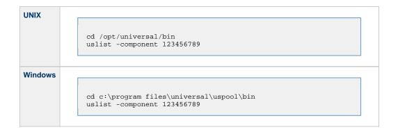
Since the -list option is not supplied, these examples, by default, list the contents of the Universal Broker Component database (UBROKER).
