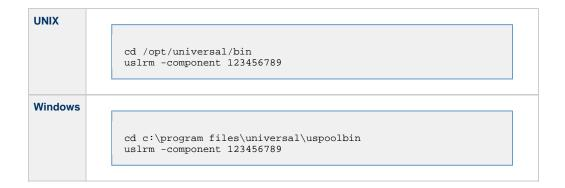
The only required option is -component (the component ID; you can execute Universal Spool List (USLIST) utility to find specific component IDs.
