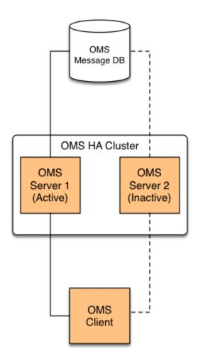
The diagram above illustrates a simple HA cluster configuration. It consists of two OMS Servers deployed on two different machines. *OMS Server 1* is the active OMS Server and *OMS Server 2* is the inactive OMS Server. Both OMS Servers share a common OMS message database. The OMS clients connect to the active OMS Server.
