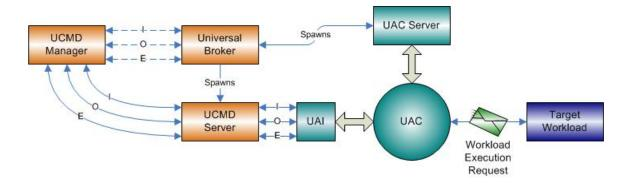
As you can see, Universal Command Agent for SOA gets its input from Universal Command through STDIN. When the parameters and data are passed in, the workload execution request is processed and any return data is passed back to Universal Command.
